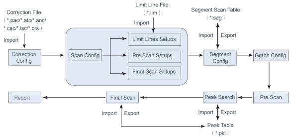
**Correction Config** Load and select the correction file; compensate the gain or loss of the external devices (such as the antenna and cable). You can view the correction data in the Correction Preview.
