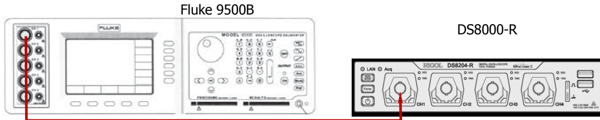
Figure 2-1 Impedance Test Connection Diagram
