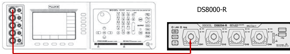
Figure 2-3 Bandwidth Test Connection Diagram
