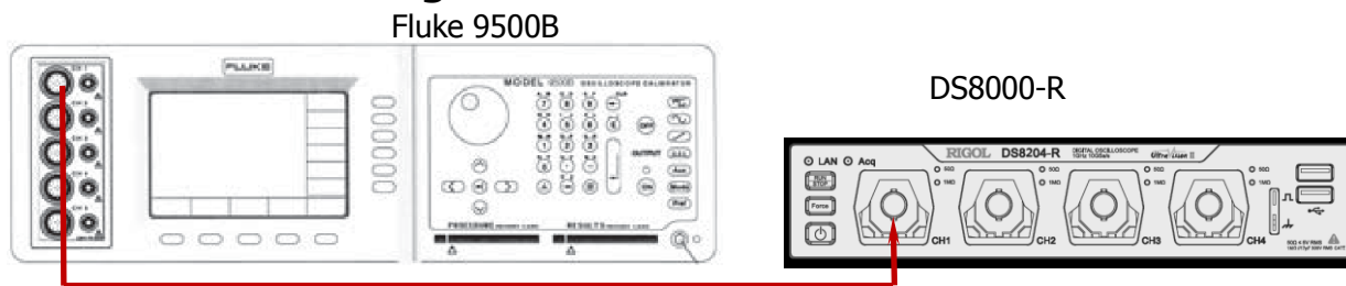
Figure 2-4 Bandwidth Limit Test Connection Diagram
