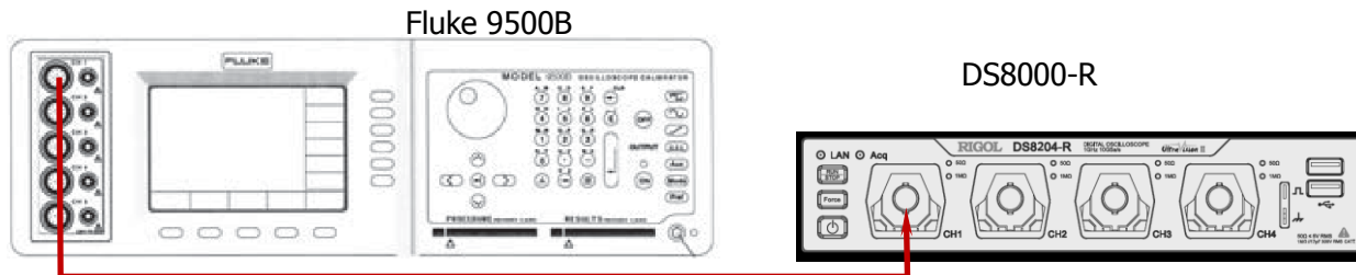
Figure 2-2 DC Gain Accuracy Test Connection Diagram
