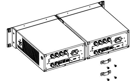
5. Mount the assembled instrument and rack into a standard 19-inch cabinet using four M6 pan head screws and four M6 square nuts.
