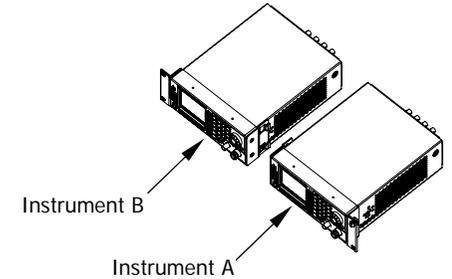
4. Place two retaining brackets onto the connecting position of rear panels of two instruments, and then secure the retaining brackets with four M4 pan head screws.
