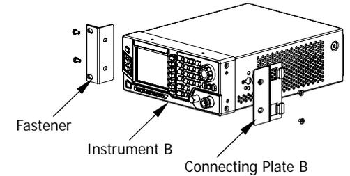
3. Join Connecting Plate A with Connecting Plate B.
